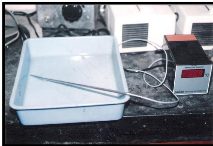
Figure: Straws being thawed at 37°C
