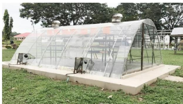
Figure 2: Parabolic shaped solar dryer
