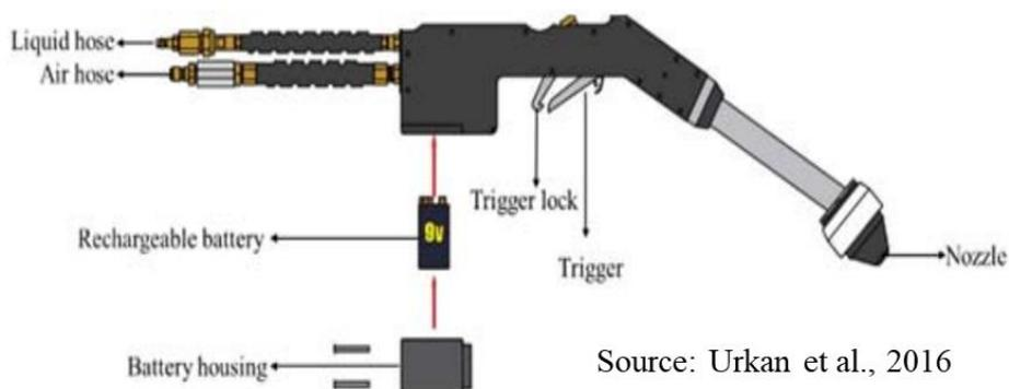
Fig. Parts of sprayer gun
