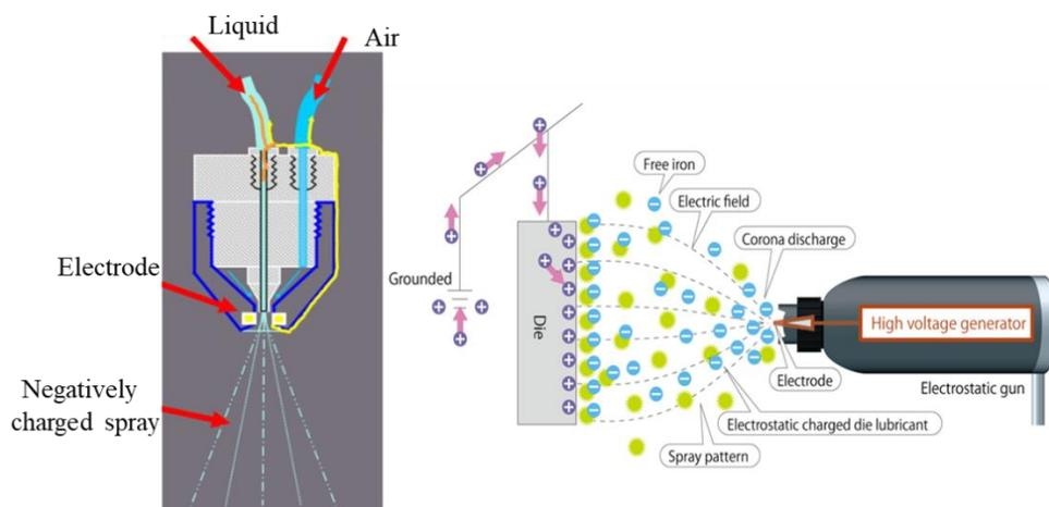
**Fig.1 Working principle of electrostatic sprayer (Source: PCB online, 2019)**
