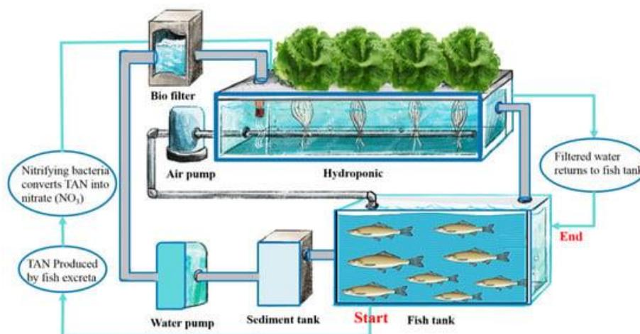
***Schematic Representation of Aquaponics (Taha et al., 2022)***
