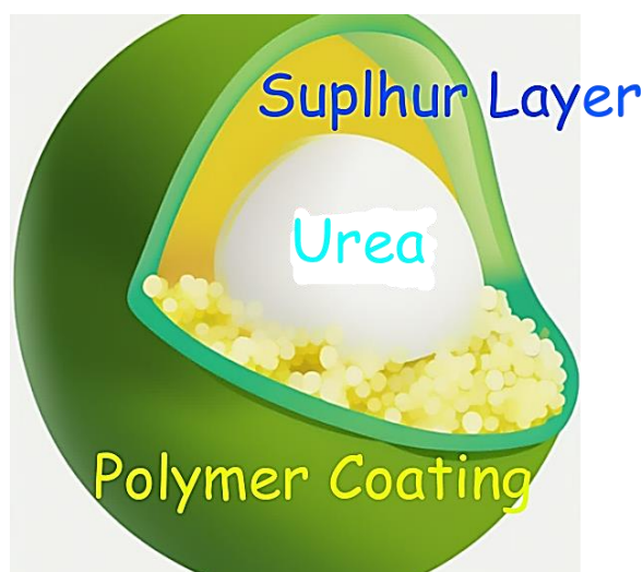
Fig:1 Layers of Sulphur coated Urea
