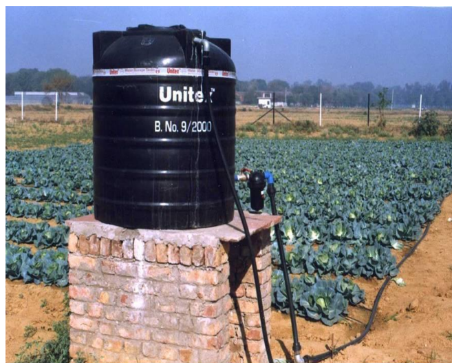
Picture 3. Low pressure drip irrigation system
