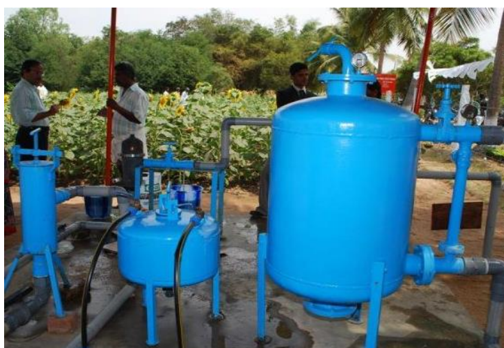
Picture 2. Micro irrigation unit for open well with Storage tank and Filter tank
