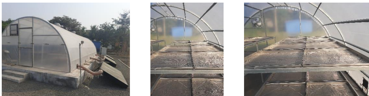
Fig. 1 Solar tunnel dryer developed at REE Department, CAET, JAU, Junagadh
