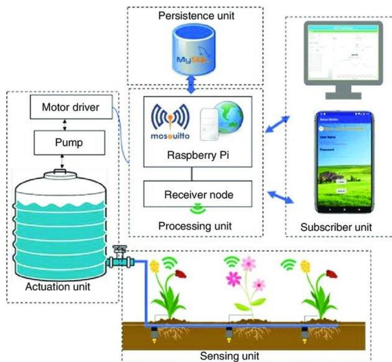
**IoT-Based Smart Irrigation System Diagram (Khriji *et al.*, 2021)**
