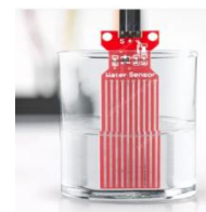
Water level sensor
